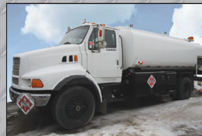
1997 FORD LS8000 FUEL TRUCK Cummins 215, 10 Spd; 16 And 23's, Almac 4 Comp't 11500L Alum Tank, Mid-Com 8000, Blackmer Pump, V/R, B/L, B620, DOT, TSSA, Stk#S-761. -1282122
