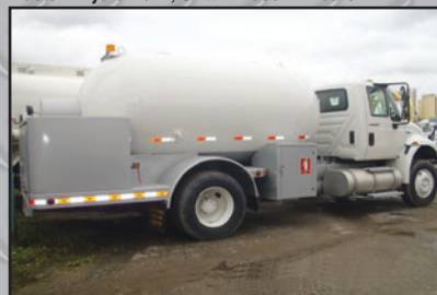
2013 INTERNATIONAL 4300 PROPANE BOBTAIL 2500 USWG, LCR, Full Refurb, New 5 yr/1 yr Inspect, Weights/Measures Calibrated Meter, TSSA Inspect, Paint Your Specs, Truck w/New DOT Inspect/Cert. Stk#S825 502045
