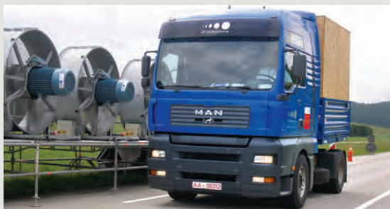
The crosswind from these huge fans had no effect on this MAN's directional stability thanks to the ZF Servoactive system we tested back in 2006. We suspect that Volvo's new Dynamic Steering system is based on that same technology.
