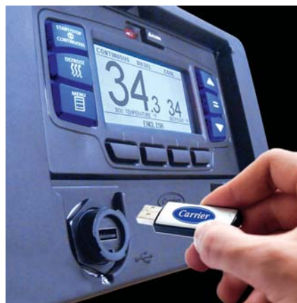
◀ Carrier Transicold's entirely new APX (pronounced 'apex') control system uses 'distributed' electronics, a first.
