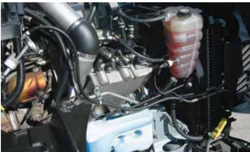
▲ AIR APPARENT: The aluminum unit above the windshield washer bottle is the first of two intake air intercoolers.
