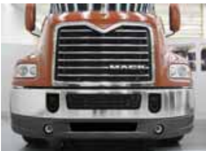
BUMPER SHOT: The molded air dam in the bumper will improve airflow to cooling package in 2007. The hood profiles remain unchanged.
