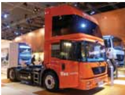
On display at the RAI show was this Mercedes-Benz Eonic tractor with a custom-built rooftop sleeper. It's powered by a quiet and efficient natural gas engine suited to urban use.
