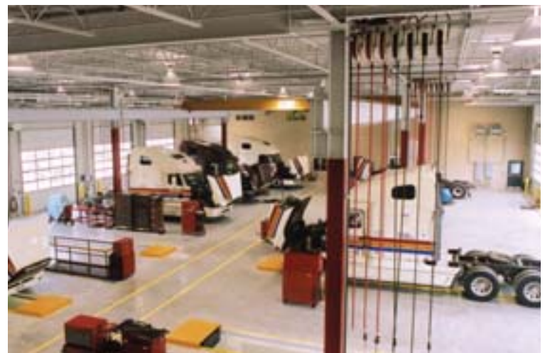
▲ The tractor repair shop runs 24/7 and can handle 12 bobtails at a time. There's an alignment rack and in a separate wing the trailer shop can do routine service on six trailers at a time plus another four needing larger repairs. Adjacent is a body shop with a 50-sq-ft paint booth. The facility is heated by waste lube oil.
