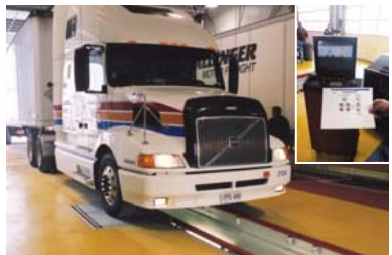
▲ When drivers finish a run, they must pull into one of three safety-inspection lanes to be fuelled. The truck's tire pressures and tire temperatures and its wheel alignment are checked automatically. Mechanics do routine maintenance in pits below, which also house a computer station and a stock of the 20 most common repair parts.
