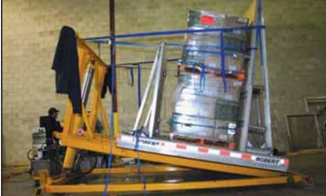
FULL TILT: Robert's tilt table invention simulates freight movements that can occur inside a van trailer.
