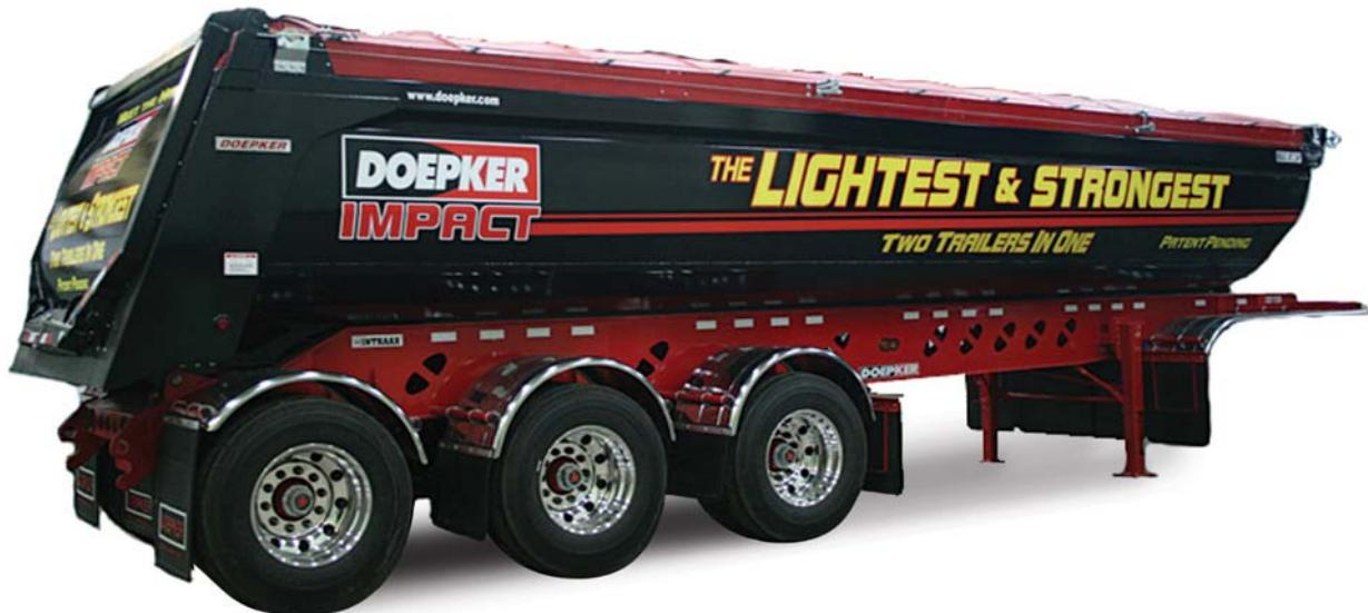
**A**fter a year of development, Saskatchewan's **DOECKER INDUSTRIES** has introduced a "highly engineered", patent-pending gravel trailer. It's claimed to be the lightest and strongest such trailer on the market with a tub made of 5/32-in., abrasion-resistant Hardox 450 plate that's said to provide significant strength combined with an extremely light tare weight. That promises maximum payload and long road life.
