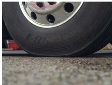
**TREADING A BIT TOO LIGHTLY:** Normally loaded, tires have a flat, even footprint. When empty at highway speed, the only center of the tread makes contact with the pavement.
