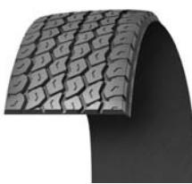
The X One XZU S retread is now available in a 390/430 tread size (the first number is the tread base width, the second the overall width, wing tip to tip). The retread is said to feature long tread life and "outstanding" scrub resistance with 23/32 original tread depth in an application-specific compound. The retread uses Michelin 'Co-EX' technology—a two-layer compound designed to minimize casing
