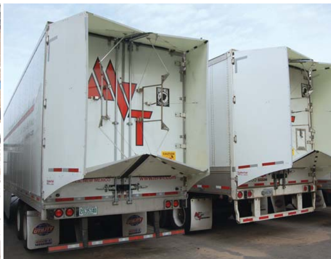
▲ TRAILER-MADE SAVINGS: Not yet legal in Canada, the ATDynamics TrailerTail is working wonders at Mesilla Valley Transportation in New Mexico. After 8 million miles of on-highway use over the last six months on 650 of the fleet's 3500 trailers, the devices have produced fuel savings of 5-6 percent.
