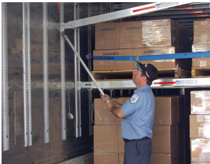
▲ THIS'LL FLOOR YOU: Ancra's Lift-A-Deck II "load maximizing system" is generating an estimated 10 to 30 percent increase in load averages while reducing freight damage claims by as much as 50 percent. That's proveable fact, the experience of Con-Way Freight, which is retrofitting its entire fleet of 16,800 vans with the Ancra product.
