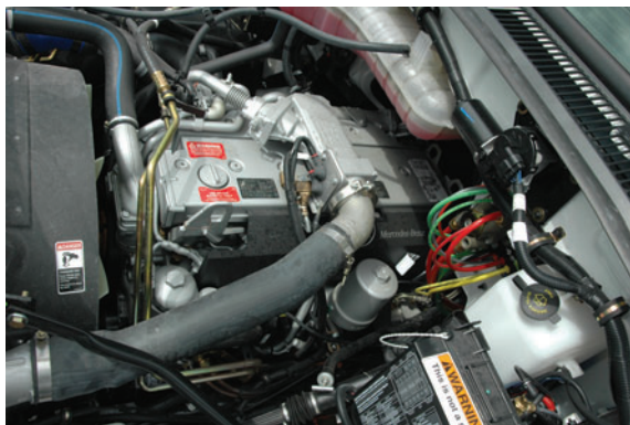
TIGHT SQUEEZE: Under the Acterra's hood, the daily maintenance items are easy enough to get at—including the main electrical panel, but keep some Band-aids around the shop for the skinned knuckles following bigger service jobs.
