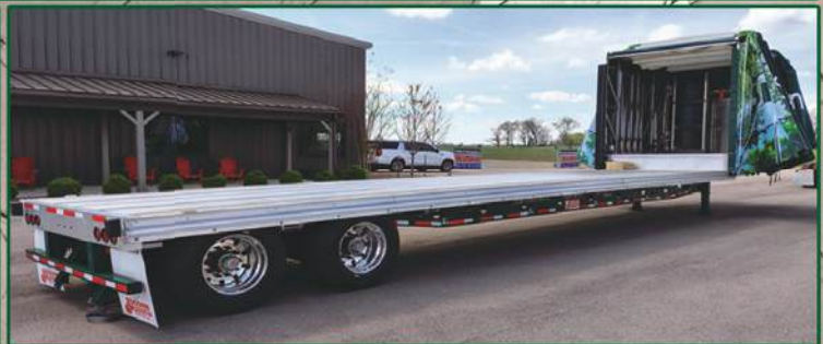
Dual Transition LCS Western Wagon Step Deck Rolling Tarp System provides loading versatility in both directions
