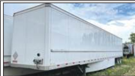
2022 DI-MOND 53' TANDEM AXLE DRY FREIGHT VAN AIR RIDE SUSP; LOGISTIC POSTS, ALUM. ROOF
